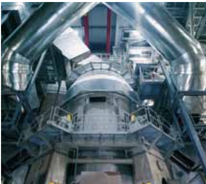
BHEL is counting on Siemens gear units to drive its vertical grinding mills.
