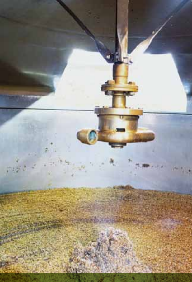
The mashing process is complicated: The mash has to be heated five times, but the temperature must never exceed 78 degrees Celsius (left). Two Roads Brewing Company (right) has relied on the Braumat Compact system from Siemens since September 2012.
