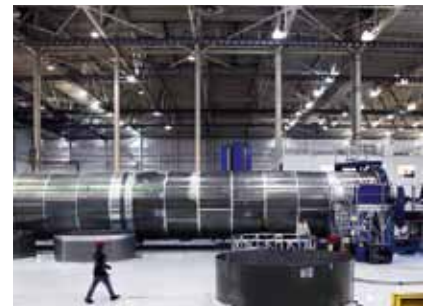
SpaceX builds complete rockets, from propulsion units to software, including large tanks.
